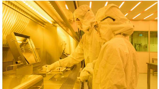
The 8,500-square-foot clean room in the UD Nanofabrication Facility is divided into Class 100 and Class 1000 spaces.
